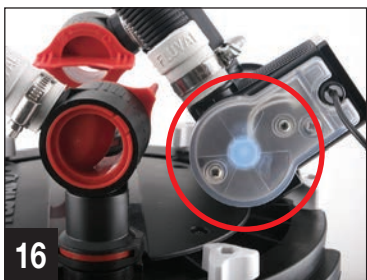
16. Ensure water is flowing out from filter. Once completed, connect power supply to UVC unit and plug into electrical outlet. A light indicator (visible through the semi-transparent lamp cover) will show that the UVC unit is operating.
