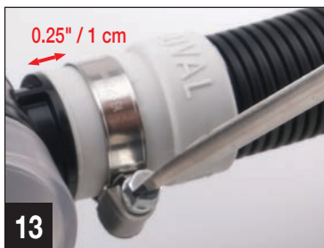
13. Double check all metal clamps are positioned approx. 0.25" / 1 cm from ends and are tightly secured with a screwdriver to ensure watertight seal.
